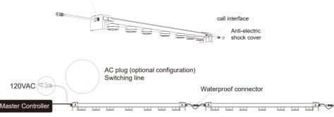
Adopting the configuration of serial RJ14 dimming cord to realize the group control
