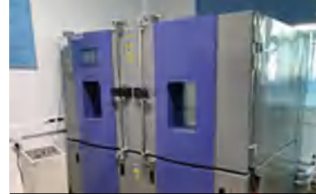
Constant Temperature and Humidity Test Chamber
