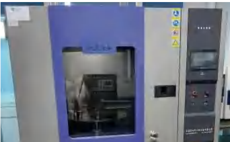
IP65 IP66 Water Spray Test Chamber
