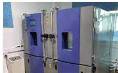
Constant Temperature and Humidity Test Chamber
